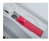
Lockswitch The Scout can be locked into a specific configuration using the lockswitch
